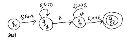
Figure 3.1: A PDA recognizing  $\{0^n 1^n : n \ge 0\}$ .
