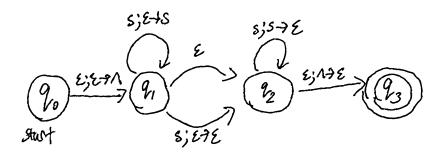
Figure 3.2: A PDA recognizing palindromes.
